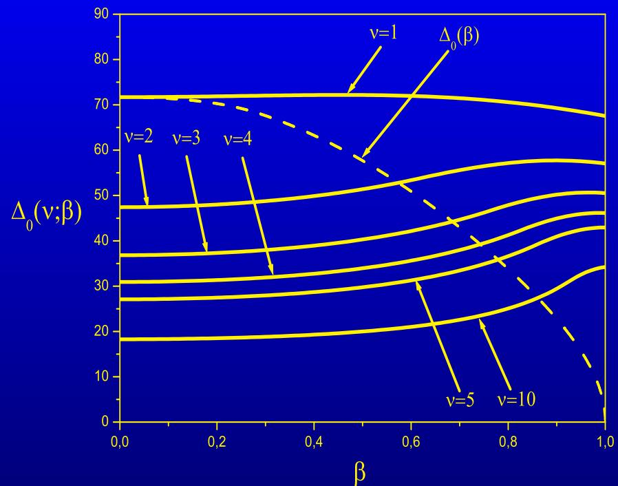
**Figure 5:** The dependence of effective angle  $\Delta_0(\nu, \beta)$  for different harmonics  $\nu$ .
