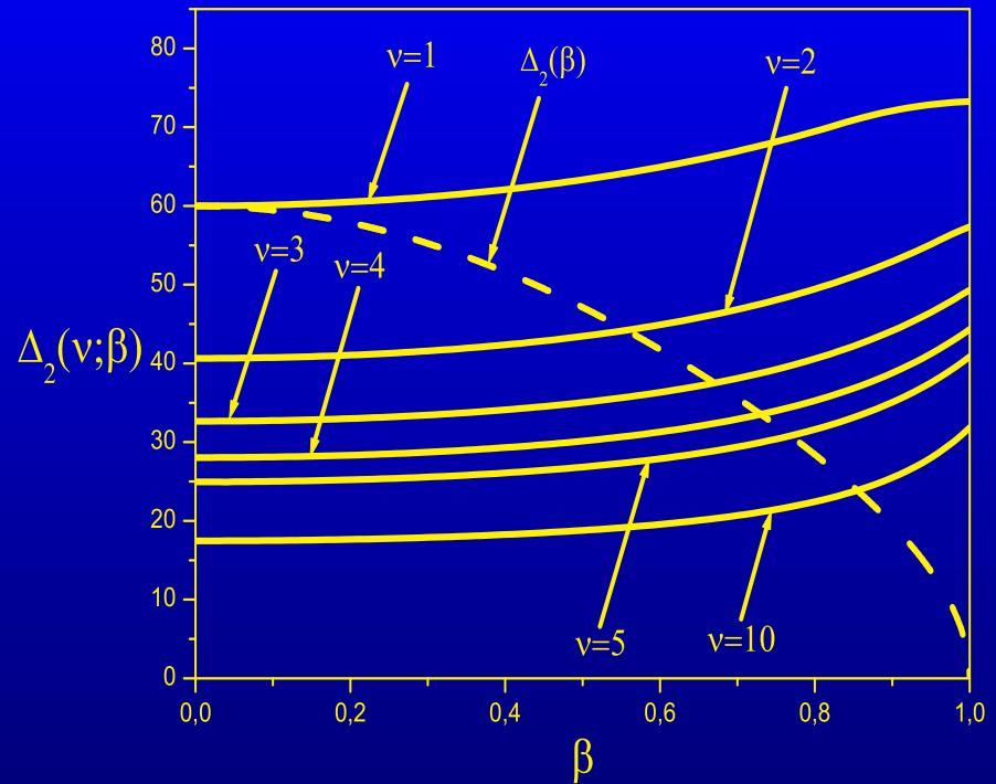
Figure 9: The dependence of effective angle  $\Delta_2(\nu, \beta)$  for different harmonics  $\nu$ .
