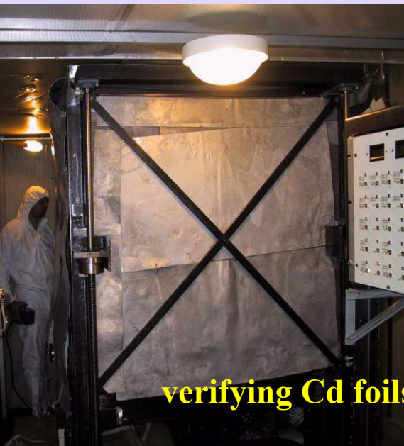
working under the passive shield before installing the paraffin
