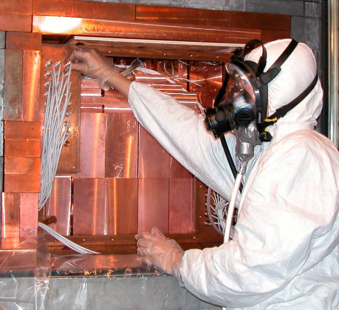
filling the inner Cu box further shield
